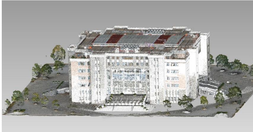
Figure 9: Fusion point cloud of Three-dimensional laser scanner and UAV tilt photography.
