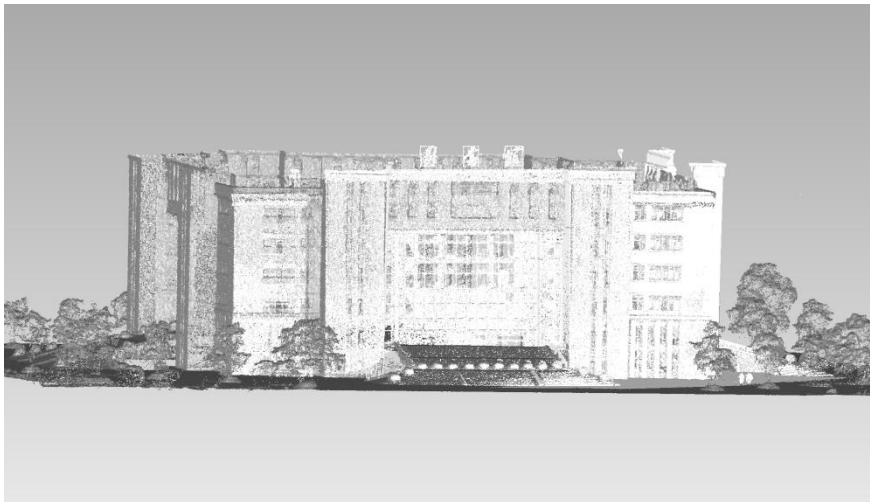
Figure 3: Registration and noise removal results of all laser point clouds.
